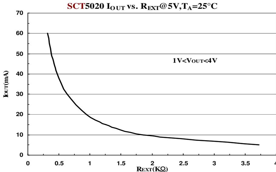
When the output voltage is larger than 1V, the constant output current set by  $R_{EXT}$  is approximate to  $I_{OUT}$  (mA) = 18.45/  $R_{EXT}$  (K $\Omega$ ). Thus the output current is about 20.5mA at  $R_{EXT}$  = 0.9K $\Omega$ .
