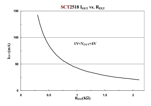
Furthermore, when SCT2518's output voltage is set between 1 Volt and 4 Volt, the output current can be estimated approximately by:  $I_{OUT} = 68(660 / R_{EXT})$  (mA) (chip skew < ±6%). Thus the output current is set to be about 50mA at  $R_{EXT} = 900\Omega$ .
