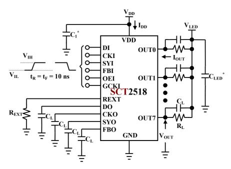
\*Place C<sub>1</sub>/C<sub>LED</sub> as close to IC VDD/OUT pin(not supply source) as possible.
