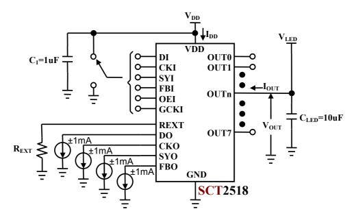
\*Place C<sub>1</sub>/C<sub>LED</sub> as close to IC VDD/OUT pin(not supply source) as possible.
