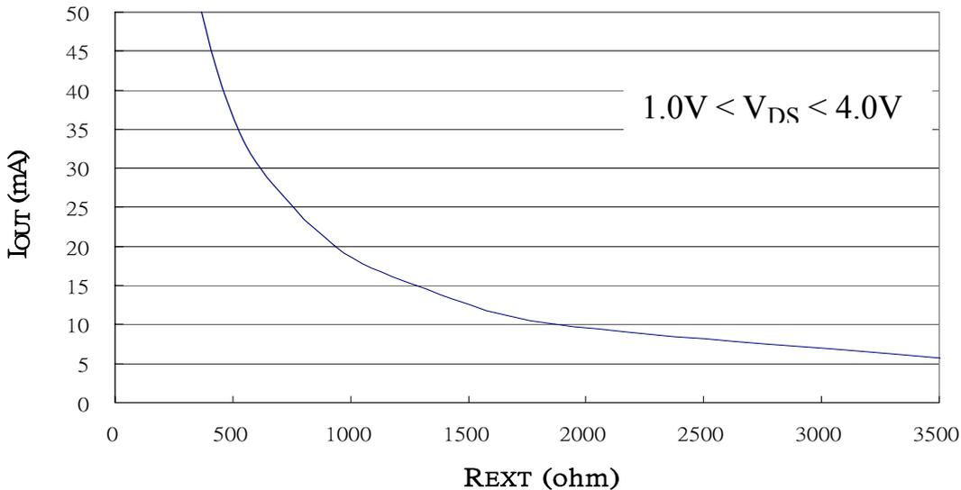
Also, when SCT2512's output voltage is set between 1.0 Volt and 4.0 Volt, the output current can be estimated approximately by:  $I_{OUT} = 30(620 / R_{EXT})$  (mA). Thus the output current are all set to be about 20.6mA at  $R_{EXT} = 900\Omega$ .
