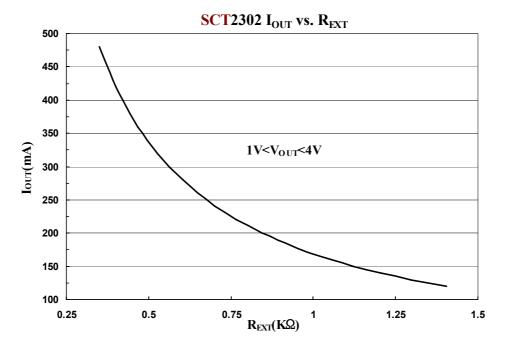
Furthermore, when SCT2302's output voltage is set between 1 Volt and 4 Volt, the output current can be estimated approximately by:  $I_{OUT} = 272(630 / R_{EXT})$  (mA) (chip skew < ±4%). Thus the output current is set to be about 190mA at  $R_{EXT} = 900\Omega$ .
