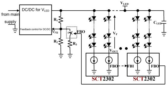
Starchips' patented multiple chips logical feedback
