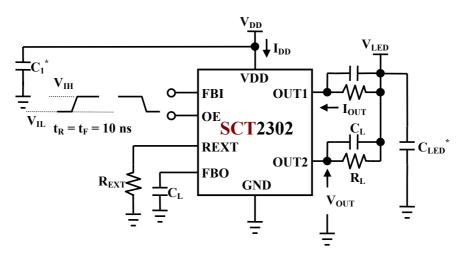
\*Place  $C_1/C_{LED}$  as close to IC VDD/OUT pin(not supply source) as possible.
