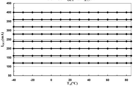
SCT2302 I<sub>OUT</sub> vs. T<sub>A</sub>@5V
