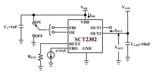
\*Place C<sub>1</sub>/C<sub>LED</sub> as close to IC VDD/OUT pin(not supply source) as possible.
