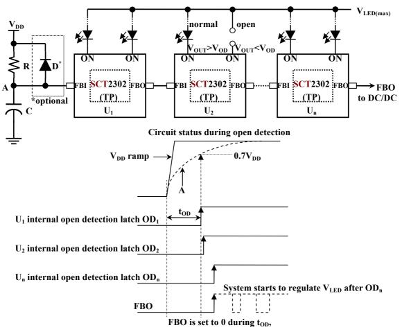
V<sub>LED</sub> is boosted gradually to V<sub>LED(max)</sub>.
