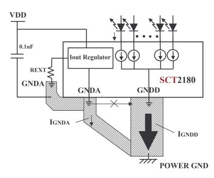
When split the ground connections, note that GNDD traces should be made shorter and wider. Maximizing the width and minimizing the length improves efficiency and ground bouncing by reducing both ground parasitic resistance and inductance. GNDA trace can be relatively narrow in application of SCT2180.
