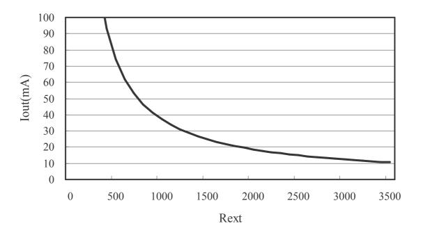
Also, when SCT2180's output voltage is set between 1.0 Volt and 4.0 Volt, the output current can be estimated approximately by :  $I_{OUT}$  =  $60(620 \, / \, R_{EXT})$  (mA) Thus the output current are all set to be about 41mA at  $R_{EXT}$  =  $900\Omega$ .
