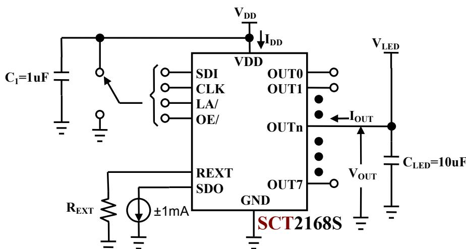
\*Place  $C_1/C_{LED}$  as close to IC VDD/OUT pin(not supply source) as possible.
