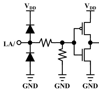
**Equivalent Circuits of Inputs (3)**
