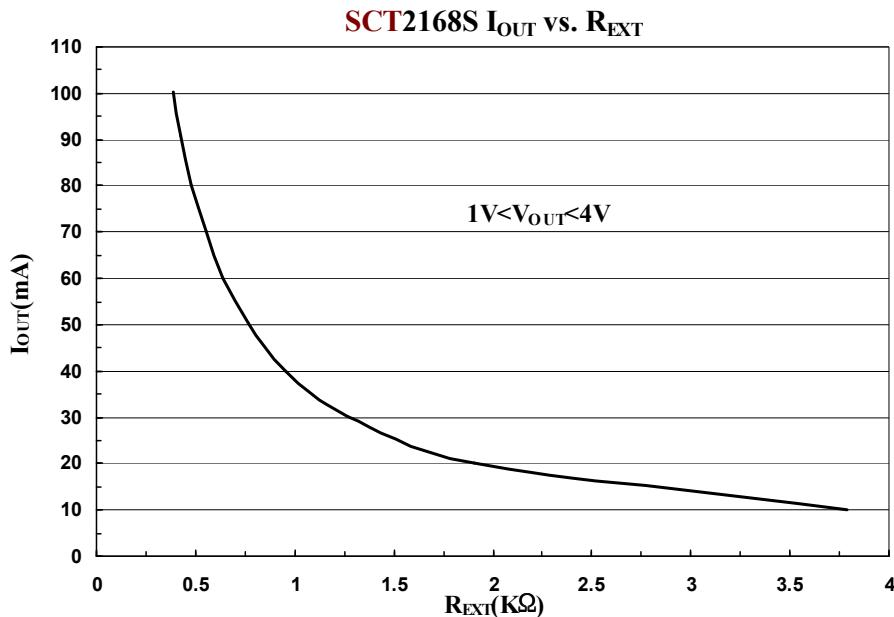
According to SCT2168S' I-V curve, the output voltage should be larger than 1V to get 100 mA constant current. By applying proper output voltage, the SCT2168S' output current set by an external resistor is approximate to:  $I_{OUT} = 60(630 / R_{EXT})$  (mA) (chip skew <  $\pm 4\%$ ). Thus the output current is set to be about 42mA at  $R_{EXT} = 900\Omega$ .
