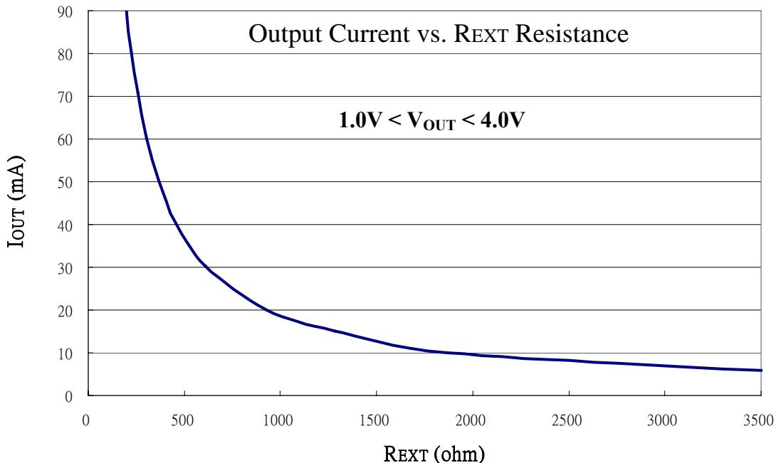
Also, when SCT2026's output voltage is set between 1V and 4V, the output current  $I_{OUT}$  can be set by the formula:  $I_{OUT} = 30(630 / R_{EXT})$  mA. Thus the output currents are all set to 20.5mA ( $\pm 5\%$ ) by set the reference value  $R_{EXT} = 900\Omega$ .
