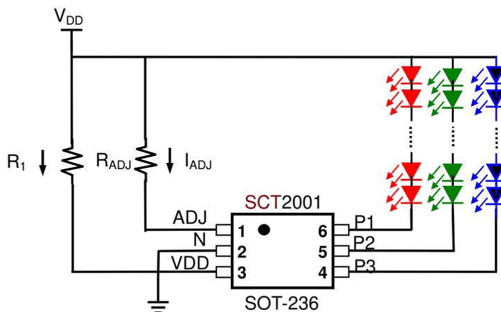
The SCT2001 can operate with wide supply input range by shunting a resistor  $R_1$  to  $V_{DD}$ . The calculation of  $R_1$  is approximately expressed by:  $R_1 = (V_{DD} - 5V) / I_{DD(max)} (1.5 \text{ mA})$ , the  $R_1$  at least 2K from supply input to the SCT2001 is required. For example, if  $V_{DD} = 24V$ , set  $R_1 = (24V - 5V) / I_{DD(max)} (1.5 \text{ mA}) = 12.5K$ . If  $V_{DD} = 5V$ , set  $R_1 = 2K$  directly.
