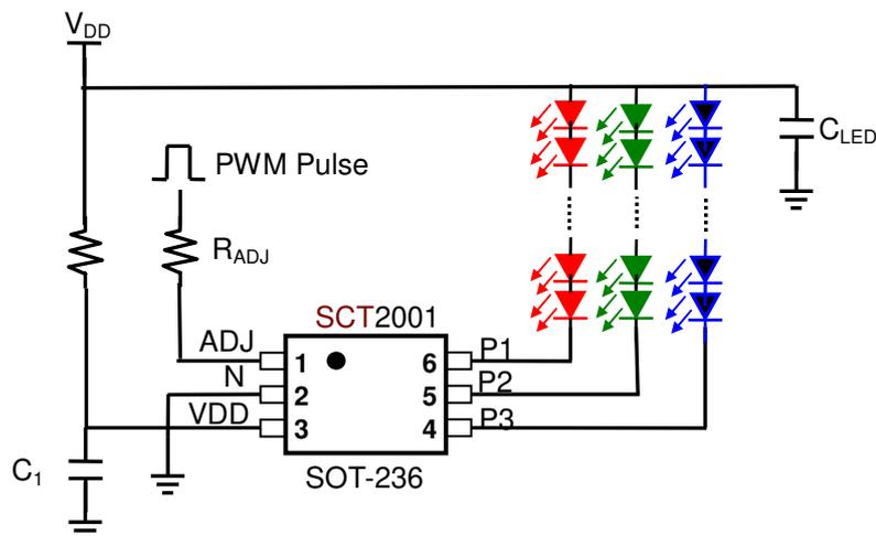
Maximizing the width and minimizing the length of  $V_{DD}$  and GND trace improves efficiency and ground bouncing. Adding a capacitor  $C_{LED}$  greater than  $10 \mu\text{F}$  beside the LED is recommended.
